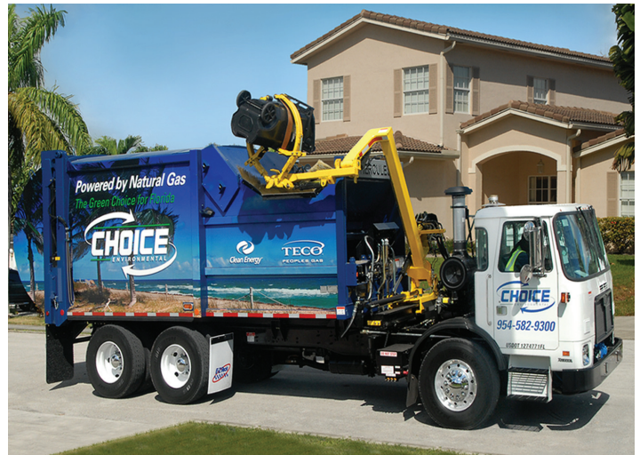
Choice Environmental Services has 11 waste collection trucks that use compressed natural gas. The trucks use chassis by Autocar LLC and Cummins Westbrock engines designed to run on natural gas power.
